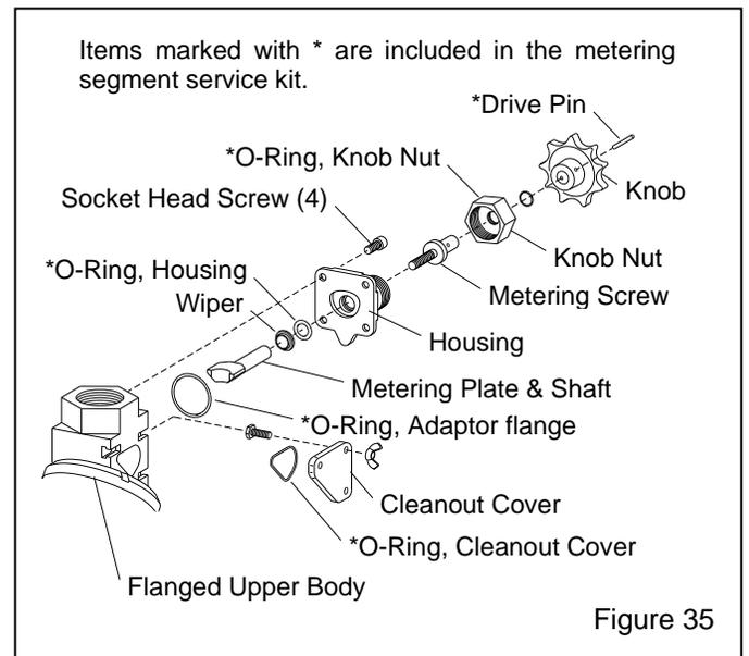
7.6.4 The flanged upper body and actuator do not need to be removed from the blast machine to service the metering assembly. Thoroughly inspect both items for wear, and replace if worn.
