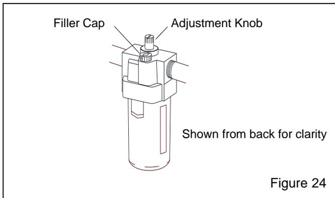
**5.5.5** Turn the adjustment knob to provide one drop of oil for every twenty strokes of the pump. If excessive amounts of oil appear to be flow through the pump during operation, as noted at the module's exhaust muffler, reduce the lubrication rate.
