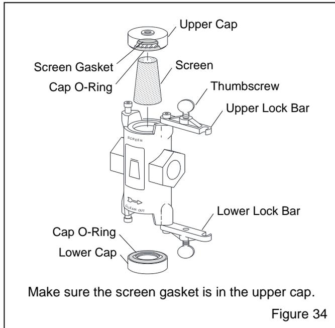
7.5.5 Install the screen in the top section. The smallest diameter end of the screen must face up, as shown in Figure 34.
