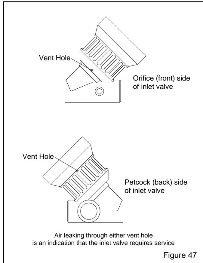
**8.6.9** Inlet valve malfunctioning. Inspect internal parts for wear, and lubrication. Refer to Section 7.3.
