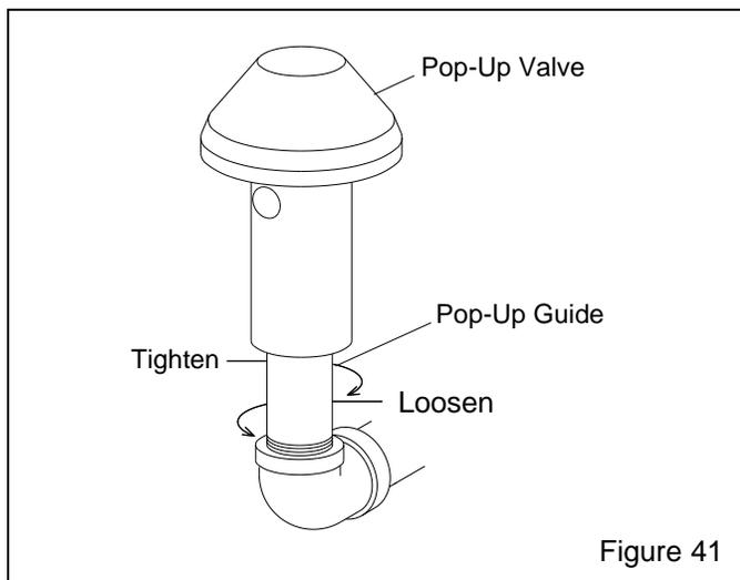
**7.9.6** While the pop-up valve is out, check alignment as follows: Screw a 1-1/4" nipple that is at least 12" long into the elbow in place of the pop-up guide. Check the alignment through the pop-up filling port. The nipple should be close to the center of the port. If it is not, adjust the horizontal pipe. A misaligned pop-up valve could result in early valve failure or abrasive leakage when the machine is pressurized or depressurized.
