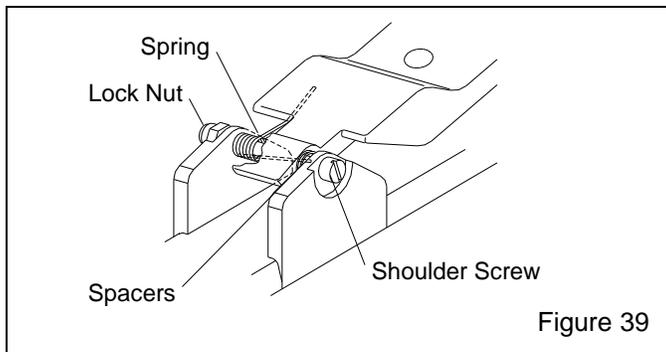
**7.8.3.3** Make sure the handle lever moves freely, raises to full up position, and does not engage unless the lever lock is pulled down.
