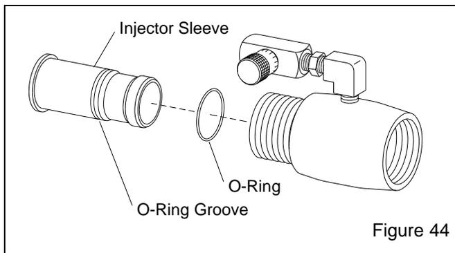
**7.11.5** Lubricate the O-ring with silicone grease or similar lubricant and fully insert the sleeve into the body.
