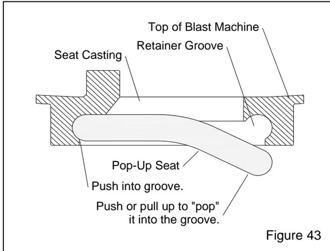
**7.10.3** Push the new seal all the way through the port and then fit it into the retaining groove. For the last few inches, pull up on the seal and allow it to pop into position.
