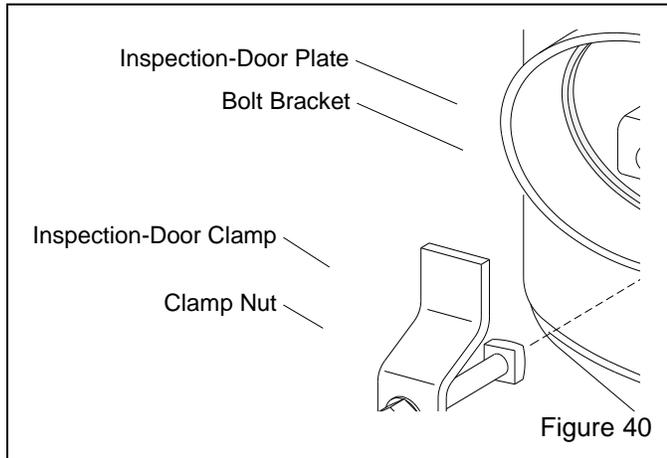
2. Push the inspection-door plate into the blast machine and rotate it so it can be removed through the inspection door. If the plate is stuck to the inspection-hole ring, rap the plate with a rubber mallet or similar tool to loosen it.
