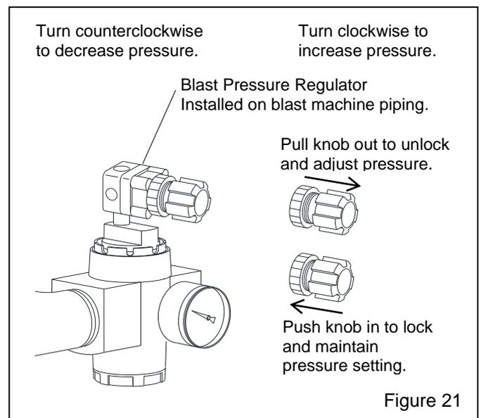
**5.2.3** If the application requires blasting below 50 psi, first pressurize the blast machine at 50 psi, and then turn the pressure to the required setting. If the initial pressure is below 50 psi, the blast machine may not pressurize.
