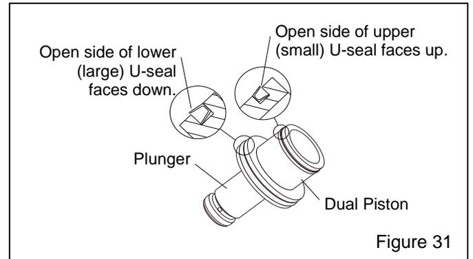
**7.3.2.6** Install the plunger and dual piston assembly into the body. Make sure the open side of the large (lower) U-seal does not fold back during assembly. The cylinder is chamfered to help slip the lip in. Tucking the lip of the seal in, while applying pressure to the piston eases assembly.
