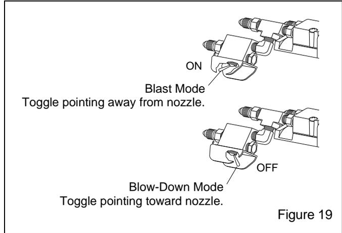
**4.6.2.2 Blow-Down Mode** Moving the ACS toggle toward the nozzle, to the "OFF" position, cuts off the control-air to the abrasive metering valve, closes the valve and stops the abrasive flow. This action allows air alone to exit the nozzle, useful for clearing the blast hose before shutting down, and blowing abrasive and water off the blasted surface.
