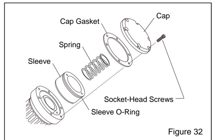
**7.3.2.8** Install the spring, cylinder cap gasket, and cylinder cap.
