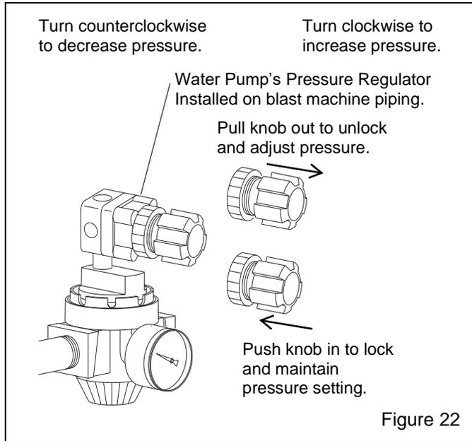
**5.3.2** Maximum operating pressure for the pump is 100 psi. The pump ratio is 10 to 1, meaning water pressure is ten times air inlet pressure. For example, if the air regulator is set at 30 psi, water outlet pressure will be 300 psi. Operating pressure is usually set between 30 and 40 psi.
