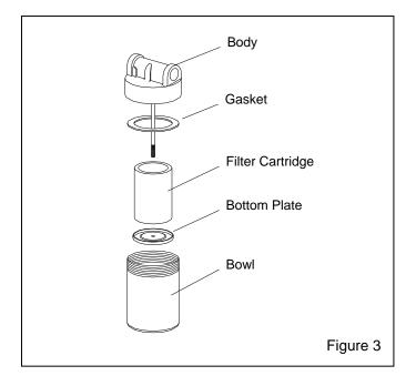
**5.2.2** Replace the cartridge at least every 200 hours of operation, sooner if a decrease of air is noted at the respirator, if pressure increases above normal at the gauge, or if the relief valve activates.
