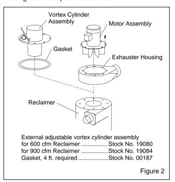
**2.1.4** Remove the backing from the gasket and place the gasket along the inside perimeter of the reclaimer bolt holes. Use cap screws to attach the vortex to the reclaimer.
