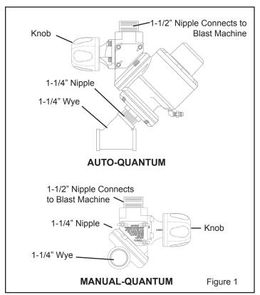
**NOTE:** The following describes installation of the Auto-Quantum valve on a machine with minimal rotation clearance. If the valve assembly will freely rotate beneath the blast machine, it may be installed as a unit.
