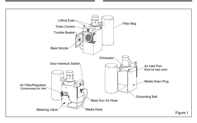
**1.9.4 Aluminum Oxide, Silicon Carbide, and Garnet:** These are the most aggressive of the commonly used media. Aggressive media may be used, but the service life of any components exposed to the media will be reduced. To avoid unscheduled downtime and maximize cabinet life, periodically inspect all parts of the cabinet, basket, nozzle, and hoses, that come in contact with the media. Boron carbide lined nozzles are recommended when using aggressive media.
