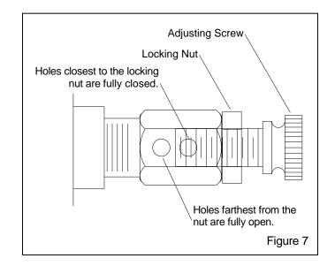
**4.3.3** If pulsation occurs in the media hose, either media is damp and caked or not enough air is entering the media stream. While blasting, loosen the locking nut and slowly turn the adjusting screw out (counterclockwise) until the media flows smoothly. Tighten the locking nut to maintain the setting.
