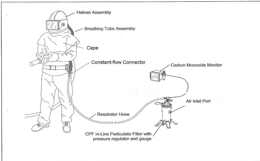
Diagram Showing a Typical Clemco Abrasive Blasting Helmet Respirator Configuration
