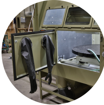
Front Access Door
