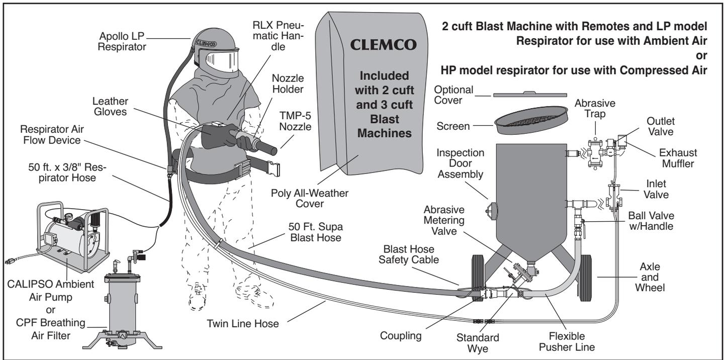
**Model 1642: 2 cuft Blast Machine, Classic with 1" piping; 150 psi working pressure**
