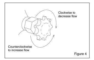
**4.1.4** Optimum abrasive flow depends on the type and size of abrasive and blasting pressure, and can best be determined by experience. Use as little abrasive as possible while maintaining the maximum cleaning rate. The air/abrasive mixture should be mainly air. As a rule, the stream of abrasive coming out of the nozzle should barely discolor the air when seen against a contrasting background.
