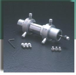
Hollo-Blast (with centering collar) for pipes 2-inch to 5-inch ID Hollo-Blast comes with a 1/2-inch short venturi nozzle and tungsten carbide deflection tip. A 5/8-inch nozzle is an option.
