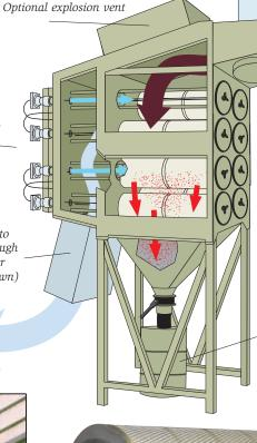
Dust-laden air is pulled into the filter housing
