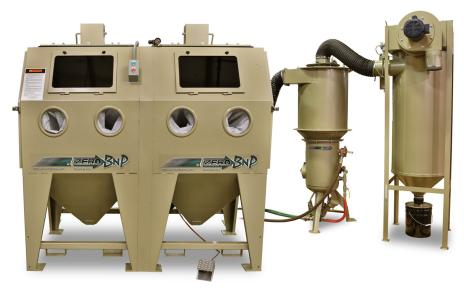
For tough cleaning jobs, pressure blasting delivers higher abrasive velocity for greater impact intensity, compared to suction blasting, and can increase your production rate by as much as 300 percent.
