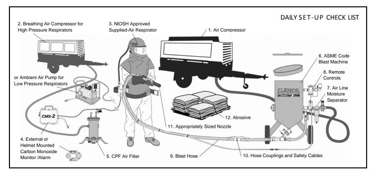
Make sure all blast operators are properly trained and suitably attired with a blast suit, safety boots, leather gloves, respiratory and hearing protection. Every day before start up, check all equipment components, including piping, fittings, and hoses, and valves, for leaks, tightness, and wear. Repair or replace as needed. Use the following checklist.
