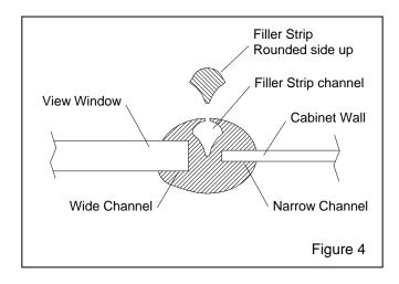
**6.** Spray silicone lubricant into the window channel (wide channel) on the molding, and slide the window into the channel, as shown in Figure 5. Place an arm into a glove to support the top edge of the bottom side of the window with one hand, while guiding the top edge into the molding with the other.
