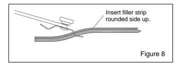
**10.** Insert the tool tip and filler strip into the filler strip channel of the molding, at the opposite side of the opening from the window molding ends, as shown in Figure 9. The rounded side of the filler strip faces up.
