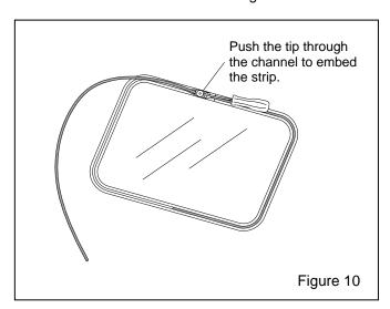
**12.** Use the window stick to push the filler strip into the molding at any spot the strip is not fully seated. Place the light-shield in its normal position.
