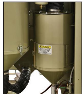
The Pulsar® suction blast cabinets combine blast, recovery, reclaim and dust collection in an efficient, compact enclosure.
