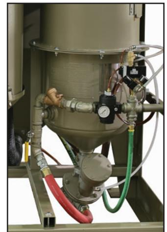
Flange-mounted blast machine on Pulsar® VIP
