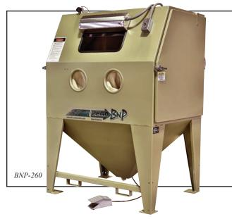
ZERO BNP Wetblast cabinets deliver affordable, dust-free media blasting to efficiently clean and finish all kinds of parts. The wetblast process produces a smooth surface, a bright shine, and does not produce static electricity commonly an issue in dry blast operations. The rinsing action produces cleaner parts than dry blast
