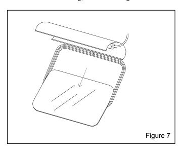
**6.3.5.** If the window molding needs replacing, replace it in the same order as the old; the narrow channel fits over the metal edge of the opening, as shown in Figure 8. The molding ends should meet in the middle of the top, straight section of the opening. Molding should be compressed so the ends are tightly sealed.
