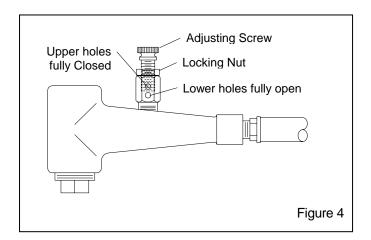
**4.3.4** If media flow is too light, decrease air in the mixture by turning the metering screw in (clockwise when viewed from the top) covering more of the holes so less air enters the media hose. Tighten the locking nut finger-tight to maintain the setting.
