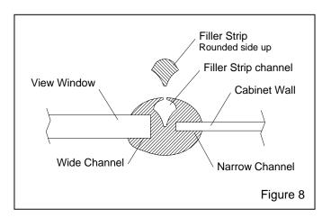
**6.3.6.** Spray silicone lubricant into the window channel (wide channel) on the molding, and slide the window into the channel, as shown in Figure 9. Place an arm into a glove to support the top edge of the bottom side of the window with one hand, while guiding the top edge into the molding with the other.
