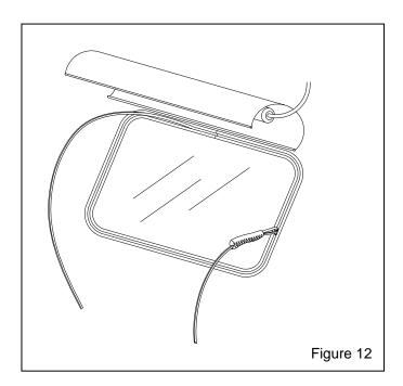
**6.3.11.** Repeat steps 6.3.9 and 6.3.10 on the other end of the filler strip. Use the window stick to push the filler strip into the molding at any spot the strip is not fully seated. Place the light-shield in its normal position.
