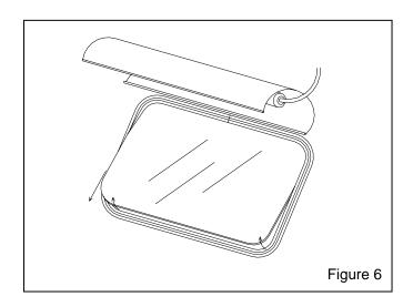
**6.3.4.** Pull the window downward to remove the window from the molding, as shown if Figure 7.
