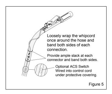
**2.2.2.2** Working from the control handle back, band the cord to the blast hose every four to six feet, and on both sides of each cord connection.
