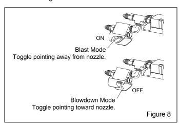
**3.5.3.2 Blowdown mode:** Moving the ACS toggle toward the nozzle, to the OFF position, cuts off the control air to the abrasive metering valve, closes the valve and stops the abrasive flow. This action allows air alone to exit the nozzle, which is useful for clearing the blast hose before shutting down, and blowing abrasive and water off the blasted surface.
