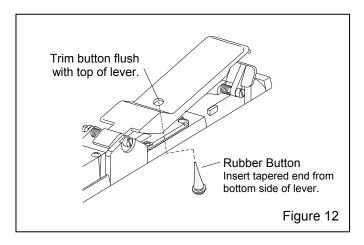
**4.6.1.3** Trim the button stem flush with top of the lever.
