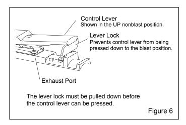
**3.2.1.2** Make sure the control lever does not seal the exhaust port on pneumatic controls, or will not engage the switch on electric controls, unless the safety lever lock is folded down.
