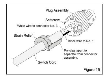
**4.7.1.5** If replacing the switch, refer to Section 4.7.3. If replacing the lo-profile connector, reassembly in reverse order, making sure the white wire goes to connector No. 3 and the black wire to connector No. 1.
