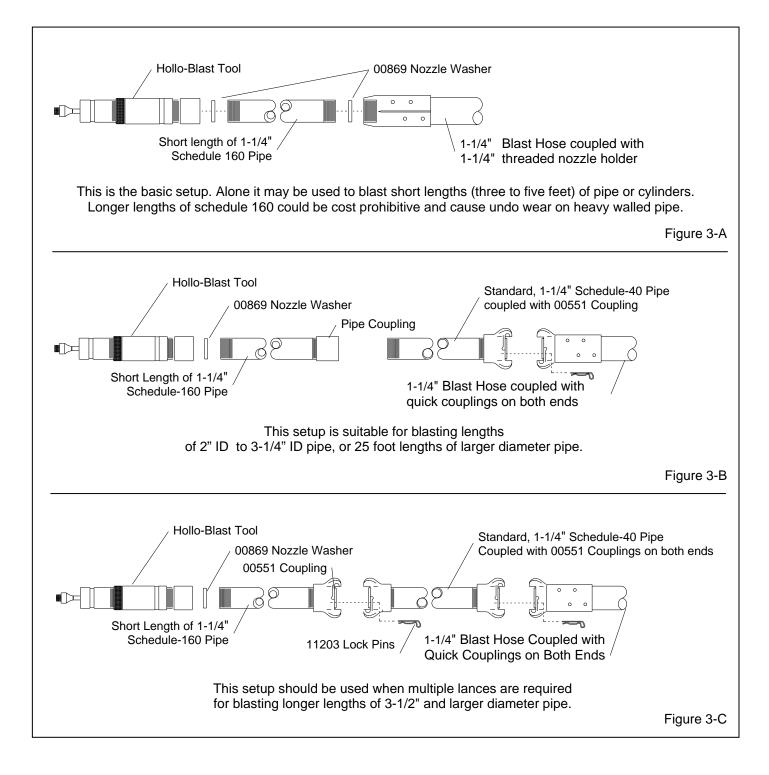
**Figure 3-A** is the basic setup; it should be used with all lance setups. Alone it is suitable for blasting short lengths (the length of the heavy-walled lance) of pipe or cylinders.
