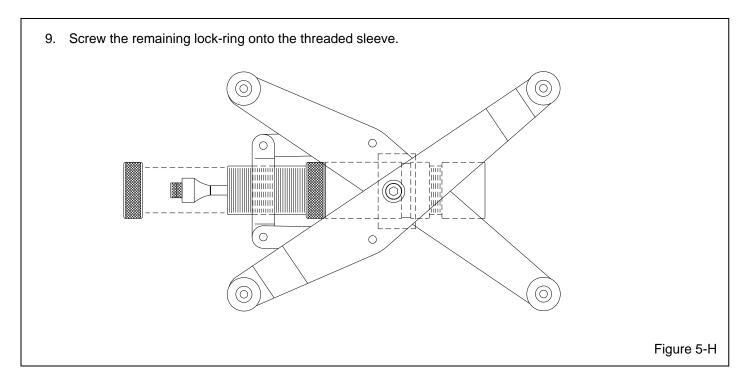
10. Adjust the carriage by turning the lock-ring onto the threaded sleeve; the farther the ring is screwed onto the sleeve, the more the carriage expands.
