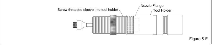
7. Screw the lock-ring tightly against the tool holder to lock the threaded sleeve.
