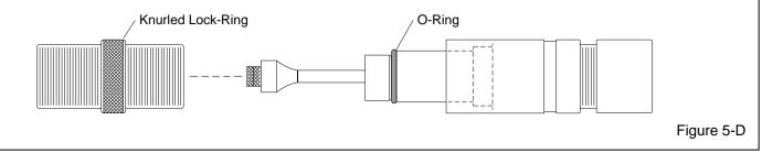
6. Screw the threaded sleeve into the tool holder until it is tightly seated against the nozzle flange. Make sure it is the sleeve that is seated against the nozzle, and not the knurled lock ring seated against the tool holder. Rapid wear on the nozzle and tool holder will occur if the tool holder is not tight against the nozzle flange.
