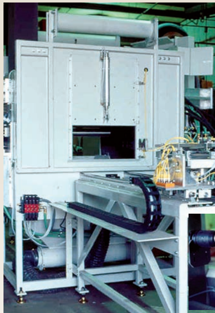
Copier rollers are prepped for coating using aluminum oxide in a fully automated blast system.
