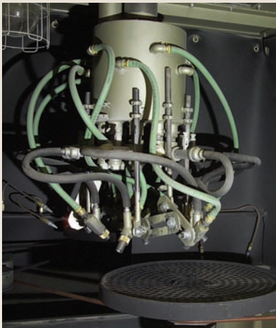
Nozzles can be easily arrayed to suit work piece processing requirements
