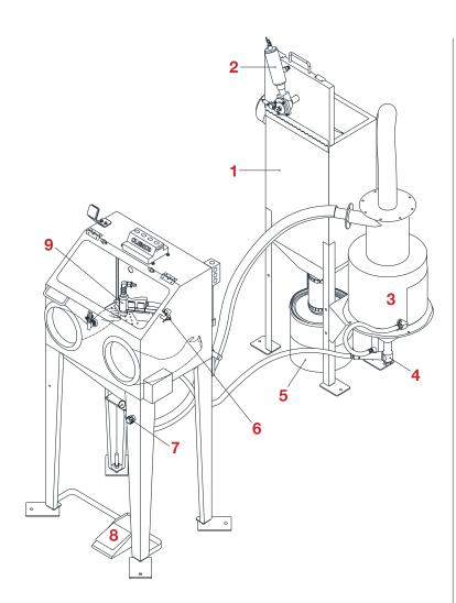
• The compact (8" diam x 16" H), vertical, topmounted cartridge can quickly be removed and replaced.
